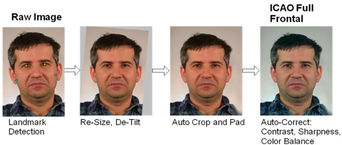
Figure 2: Cropped face image is automatically adjusted to best fit ICAO standards and best practices
